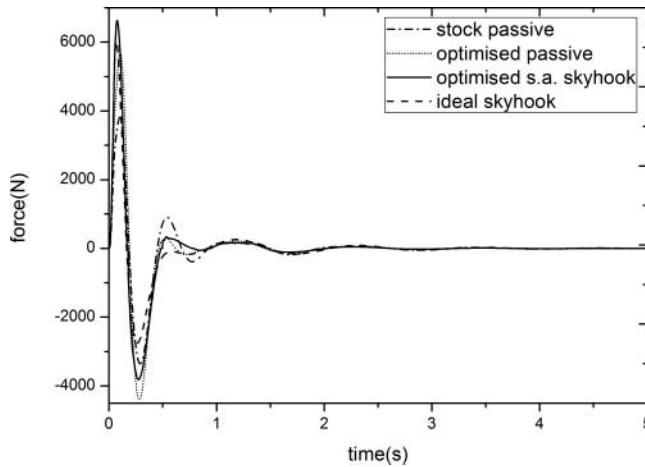
Figure 14. Time history of rear suspension damping force for a single damper in stock passive, optimised passive, optimised semi-active skyhook, and ideal skyhook suspensions.
