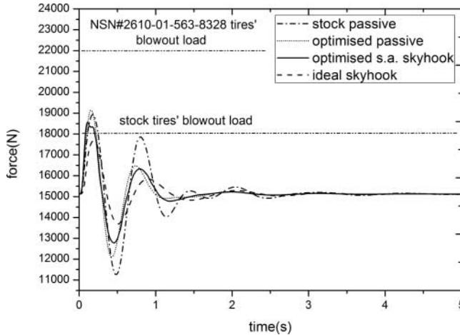
Figure 10. Time history of front tyre force with stock passive, optimised passive, optimised semi-active skyhook, and ideal skyhook suspensions.
