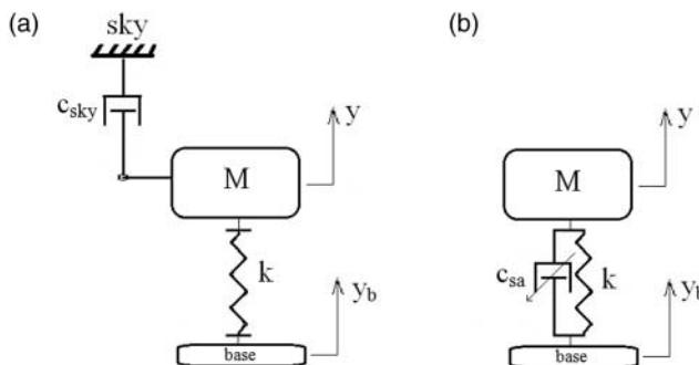
Figure 4. Schematic figure of: (a) ideal skyhook and (b) semi-active skyhook configurations.
