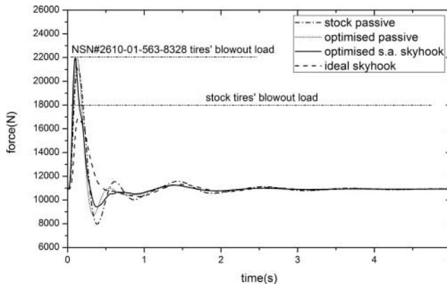
Figure 9. Time history of rear tyre force with stock passive, optimised passive, optimised semi-active skyhook, and ideal skyhook suspensions.
