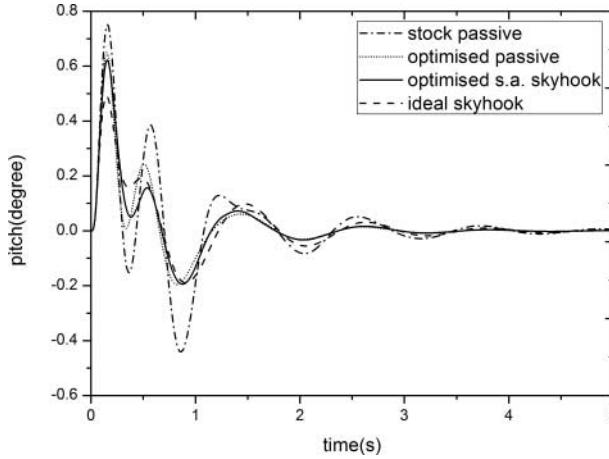
Figure 7. Time history of vehicle pitch with stock passive, optimised passive, optimised semi-active skyhook, and ideal skyhook suspensions.
