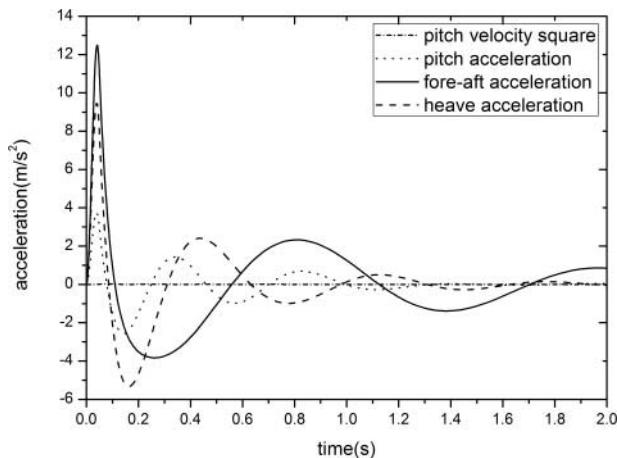
Figure 5. Comparison of order of square pitch velocity with heave, pitch, and fore-aft accelerations of the vehicle with stock passive suspension.
