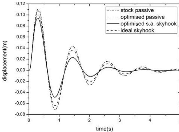
Figure 8. Time history of vehicle fore-aft motion with stock passive, optimised passive, optimised semi-active skyhook, and ideal skyhook suspensions.
