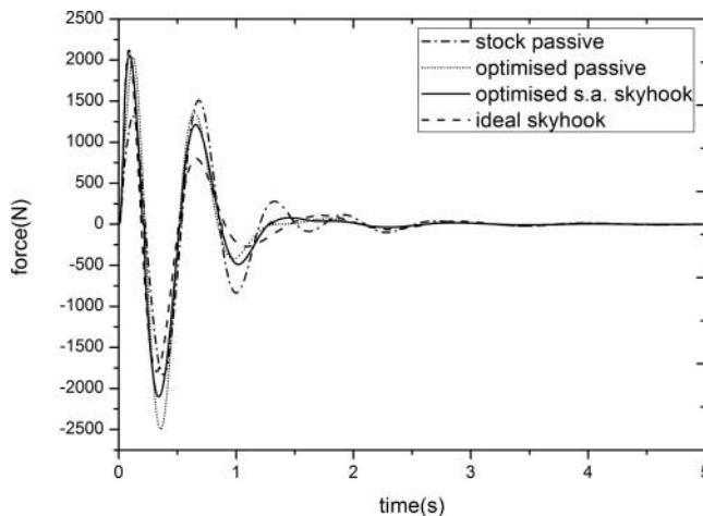
Figure 15. Time history of front suspension damping force for a single damper in stock passive, optimised passive, optimised semi-active skyhook, and ideal skyhook suspensions.
