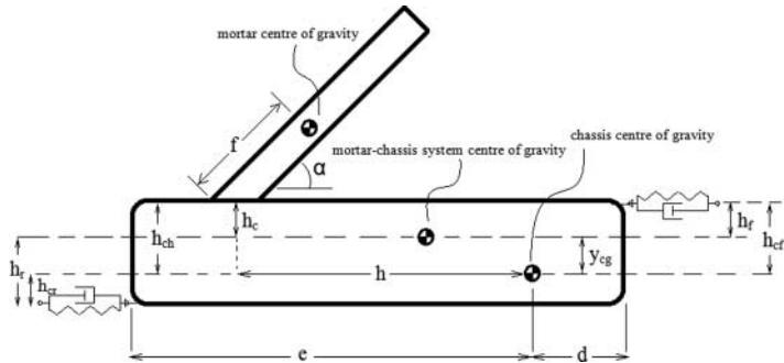
Figure 3. Multi-body mortar-chassis model.
