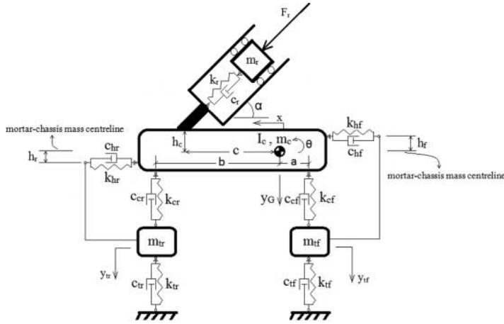
Figure 2. Schematic 2-D model of a HMMWV with mounted SRAMS.
