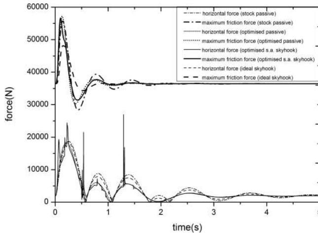
Figure 11. Time history of total horizontal and friction forces exerted on the tyres through the suspension and the ground in stock passive, optimised passive, optimised semi-active skyhook, and ideal skyhook suspensions.
