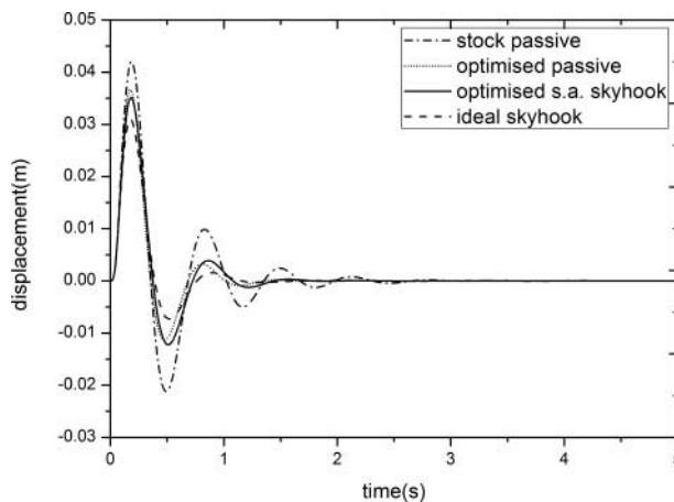
Figure 6. Time history of vehicle heave with stock passive, optimised passive, optimised semi-active skyhook, and ideal skyhook suspensions.
