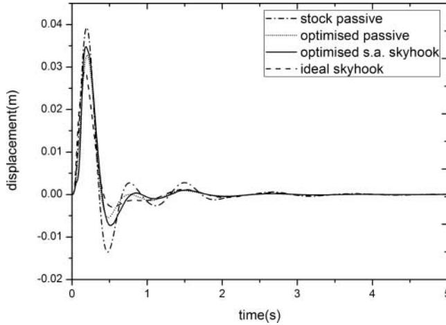
Figure 12. Time history of rear suspension travel for stock passive, optimised passive, optimised semi-active skyhook, and ideal skyhook suspensions.
