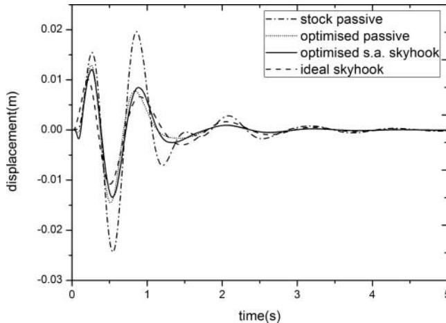
Figure 13. Time history of front suspension travel for stock passive, optimised passive, optimised semi-active skyhook, and ideal skyhook suspensions.
